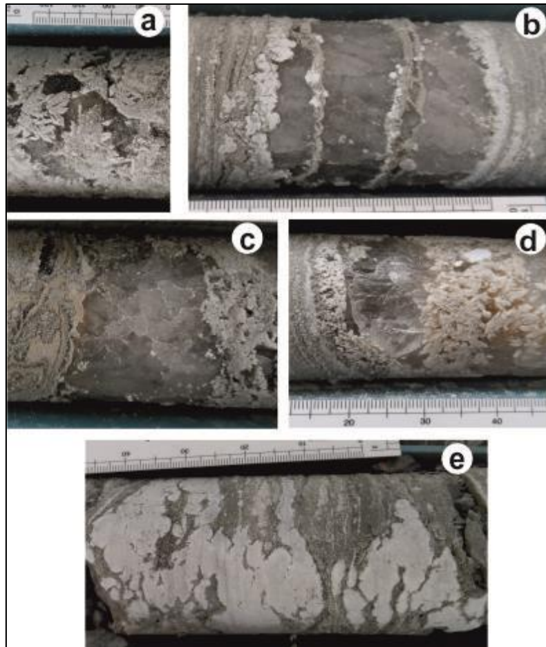
Figure 2. a) Euhedral glauberite, b) intercalation of halite, anhydrite, carbonate and aligned halite crystals, c) mosaic halite, d) halite and euhedral glauberite, e) anhydrite nodules
