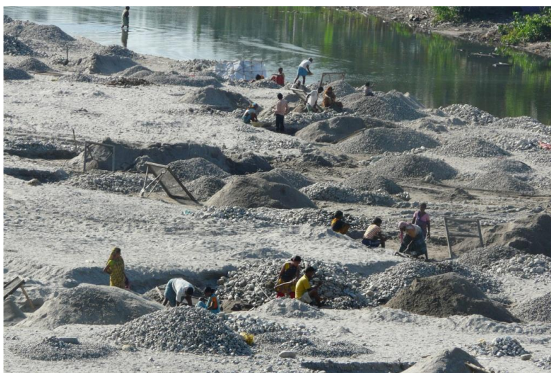
Photo 3. Bed material extraction from the Balason river by the local community (Nimtijot village)
