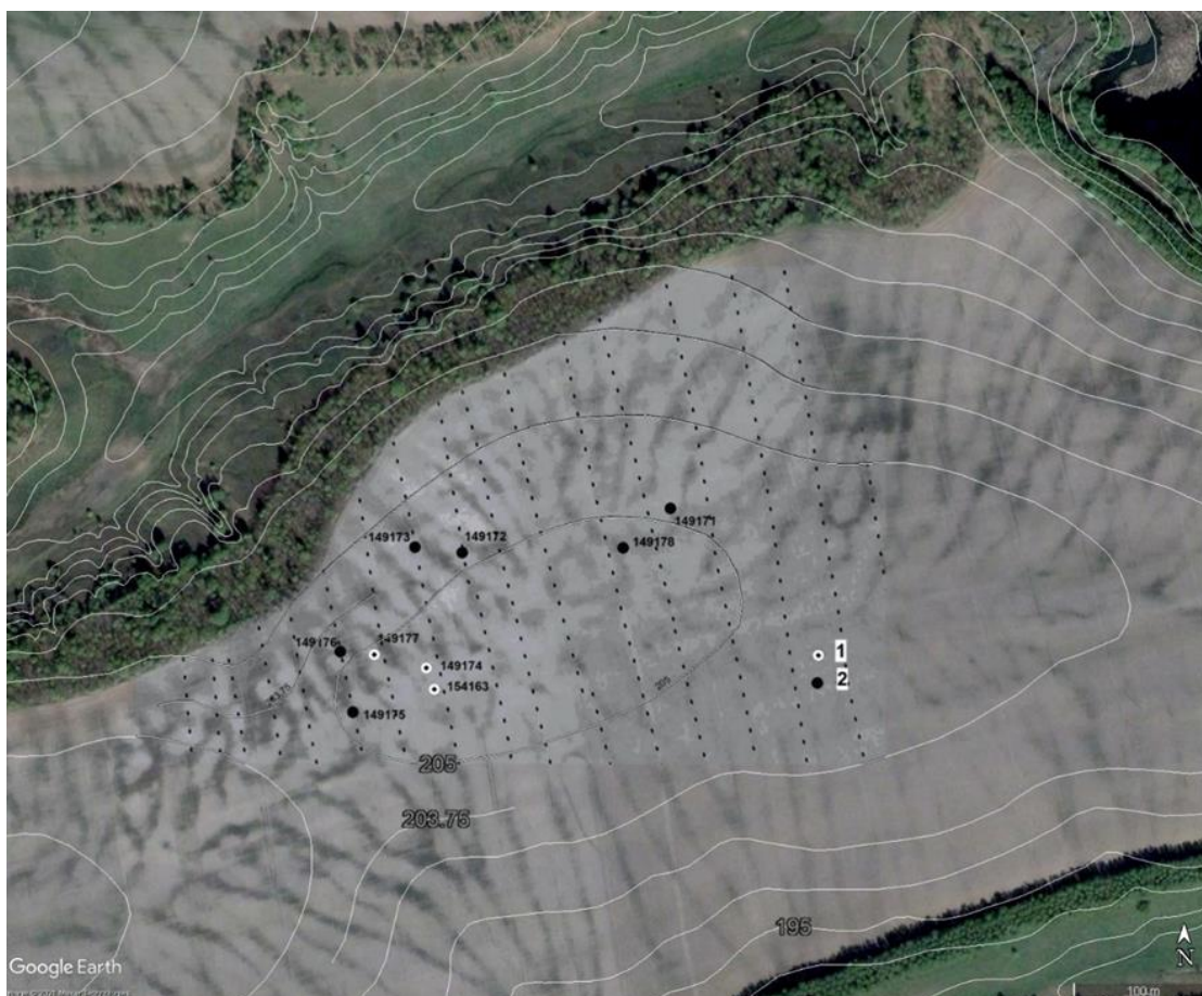
Figure 3. Soil sampling points (1 – samples to determine reference value of caesium-137 radioactivity, 2 – other sampling points); dotted lines represent locations of the plowing furrows in 2014; point 149171 is located in plowing furrow of 2003 (it is detected as a barely discernible light strip in the satellite image)
