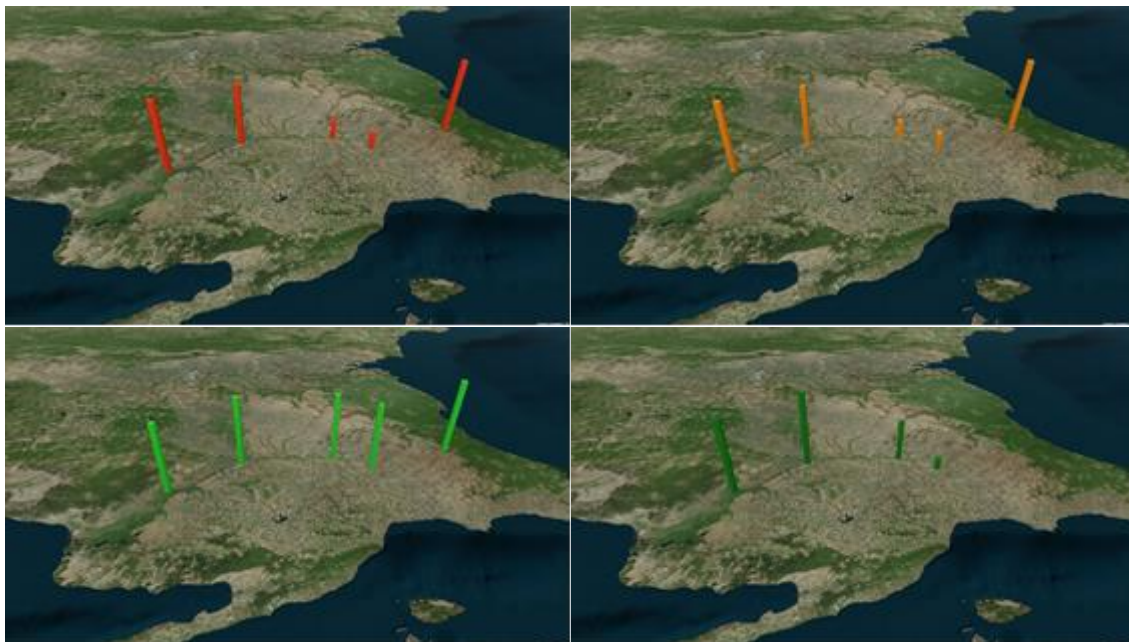
Figure 2. DO (up-left – mg/L), %O2 (up-right – %), pH (down-left – pH), turbidity (down-right – NTU) levels
