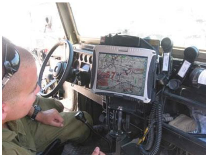
Figure 4: Integrated Communications C4I Systems For Security Applications
